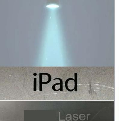
Fiber Laser is popular used for marking logo, serial number, bar code or other designs on metallic products such as bearing, gold ring, hardware tools, aluminum nameplat & consumer electronics. Also it can be used for part of engineering plastic such as keyboard, mobile charger housing, plastic toy and etc
